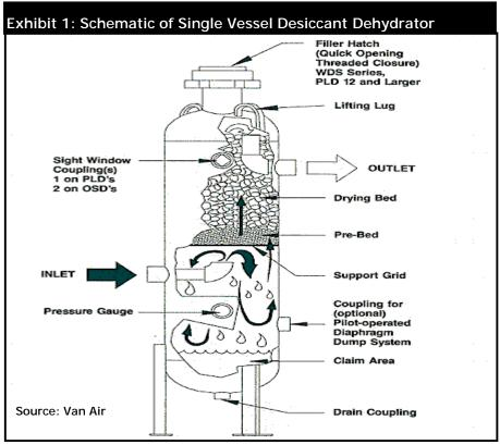
Gradually the moisture dissolves the desiccants into brine droplets, which trickle down into the claim area that is connected to a brine storage tank. When the desiccants reach equilibrium or the maximum amount of moisture they can adsorb, the 'dry' gas exits on the top of the vessel to the main gas line.
